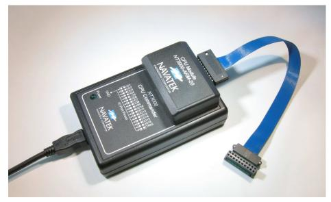
command. A built in macro language supports easy development of complex test procedures without the need to learn a programming language. For custom test systems, the NT3000 CPU Commander<sup>TM</sup> can interface to any programming language capable of supporting DLL's such as Visual C, Visual Basic, ATEasy<sup>TM</sup>, Delphi<sup>TM</sup>, LabView<sup>TM</sup> and LabWindows/CVI<sup>TM</sup>.
